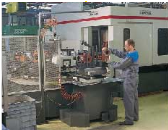
One of the flexible cells used for the machining of complex components, supplying the assembly lines on demand.
