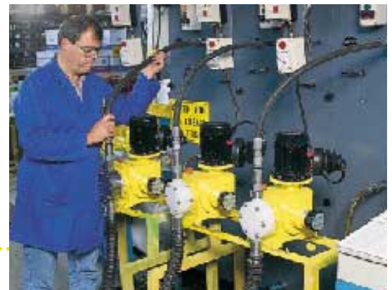
Each Dosapro Milton Roy pump is tested on an automated test bench.
