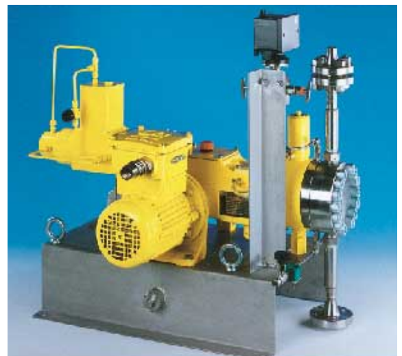
MILROYAL® D with a double diaphragm head with flushing of the double diaphragm chamber (pyrophoric products).
